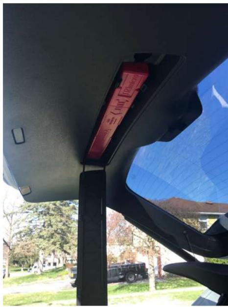
Stowing the triangle is easier, as there is a storage space made specifically for it on the trunk door. You twist open the latch, the cover drops down, and the triangle case snaps soundly into place. To remove it, you open the cover, then break off some fingernails prying the triangle out of the snaps.
