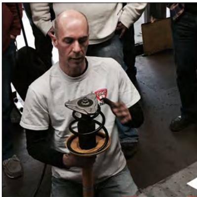
crew as why this was important, especially if you didn't want to repair your garage ceiling or visit an ER. Once compressed, the strut mount was removed via an impact wrench and a box wrench. The strut was then disassembled and reassembled with the spanking new yellow Bilstein.
