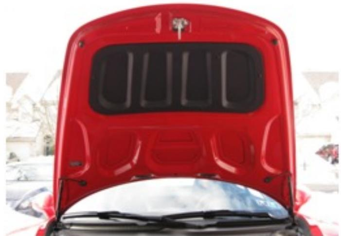
Here is the hood with the lid liner installed.
