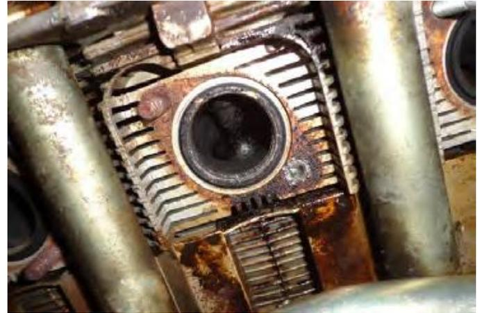
Here we have all that was left of the old rotten stud, a nice coil of threads. The result is that the original tapped threads remain in the cylinder head completely untouched. This is a very precise tool indeed.
