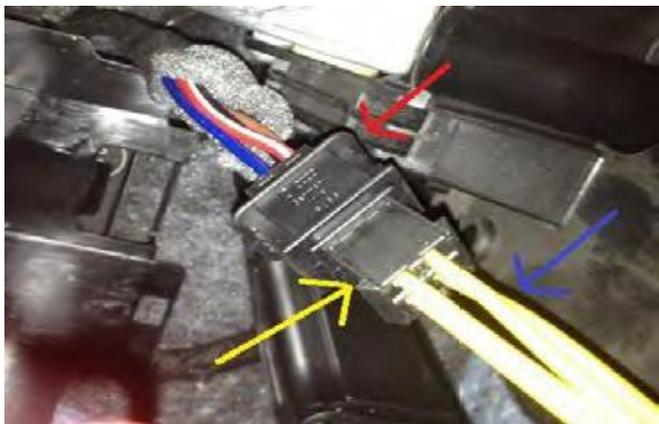
Here we have the relay wired inline from the harness to the brake controller, which is then secured out of the way up under the dash.
