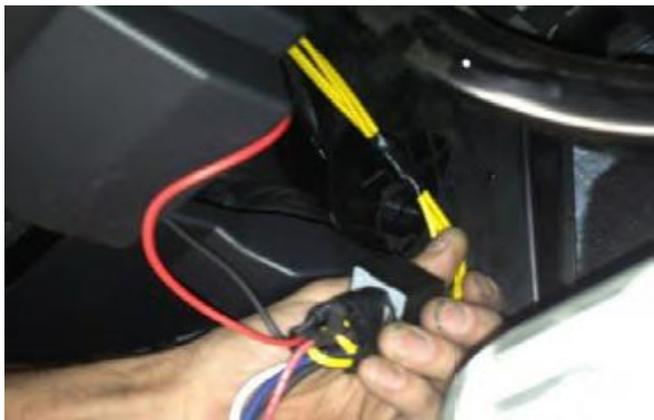
And finally, we find a place to mount the brake controller following the controller's instructions. They do need to be mounted in the direction of travel to work properly, and there are numerous locations you can use under the
